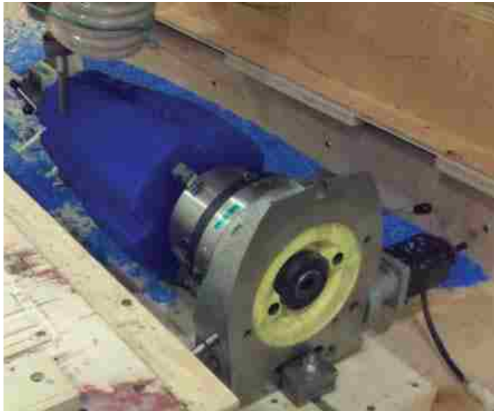
Figure 9: Part and resulting waste after CNC routing
