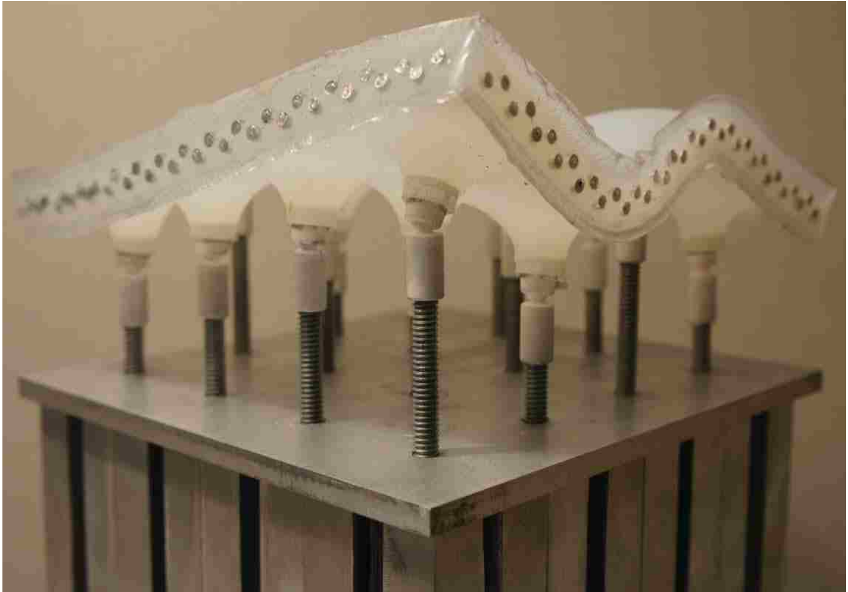
Figure 46: One forming wall from final [m]form prototype
