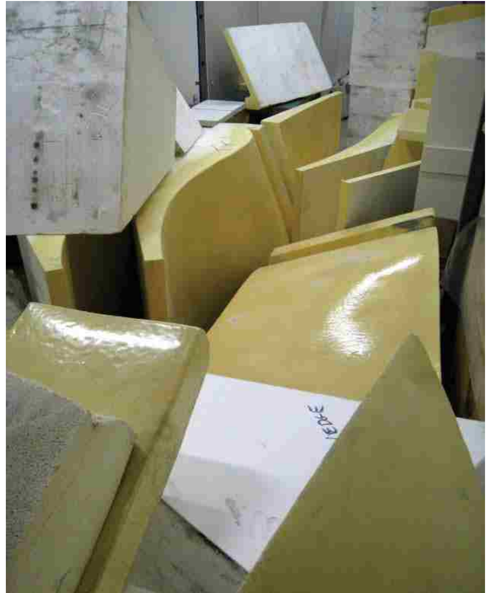
Figure 10: One-off foam molds used to form concrete ceiling/ Photo by Caliper Studio
