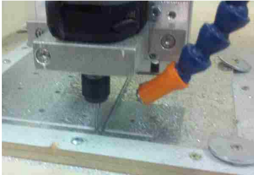
Figure 40: CNC routing fabrication of sheet aluminum wall for final prototype
