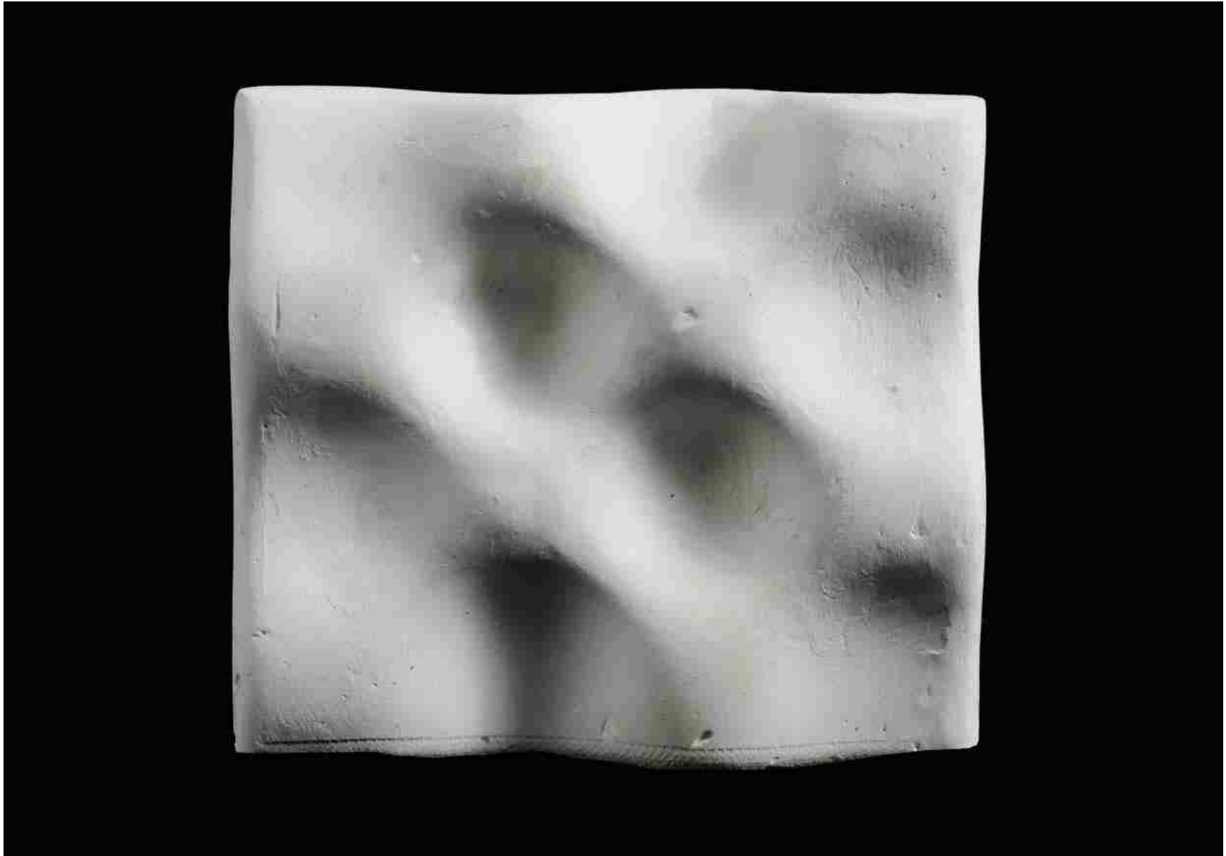
Figure 44: Cast plaster panel produced using final [m]form prototype
